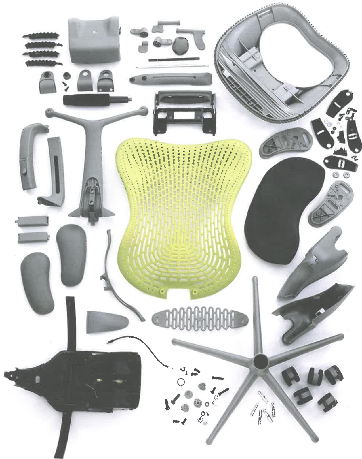
American office furniture manufacturer Herman Miller developed the Mirra® Chair, which is Cradle to Cradle Certified 'Silver'. The materials used are free of toxins and 97% recyclable. Each connection between different materials can be taken apart by one person in less than 15 seconds. For its production, the company built a new factory that runs on renewable energy and like the chair itself meets the Cradle to Cradle motto 'waste equals food'.
