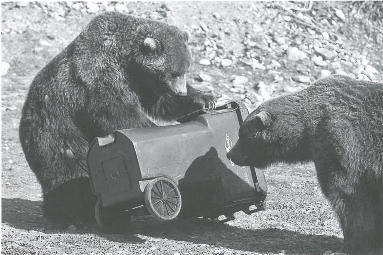
Bear-resistant containers come in all sizes and shapes, from ultra-light backpacker food containers weighing a few ounces to dumpsters able to hold 20 tons. Some of these products have been tested by trial and error through direct experience with bears, and actually meet the criteria for 'bear-resistance'.
