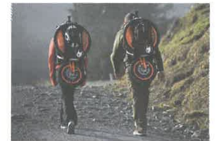
How to make a bicycle portable? Dutch bicycle manufacturer Koga developed the Bergmönch, a compact mountain bike that can be carried like a rucksack for hiking uphill and wheeling downhill.
