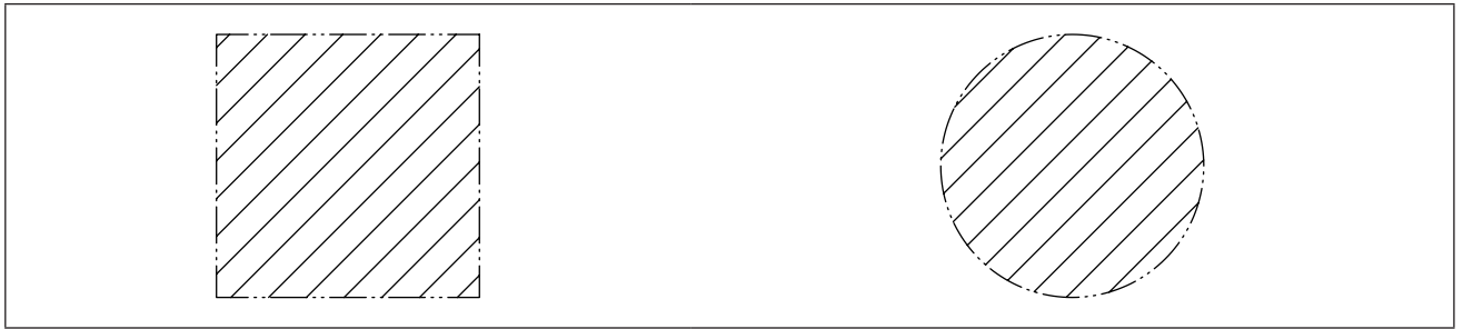
Figure 101 – Datum target area
