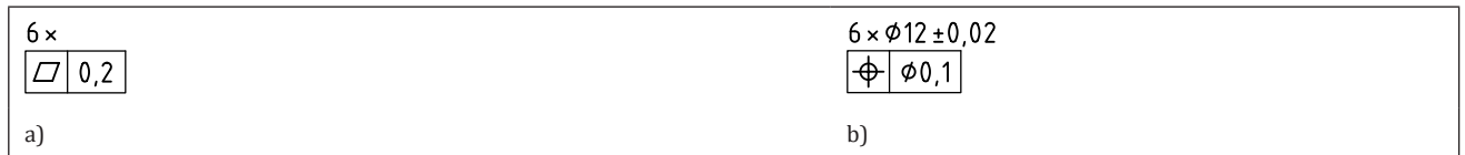
Figure 122 – Tolerance applying to more than one feature
