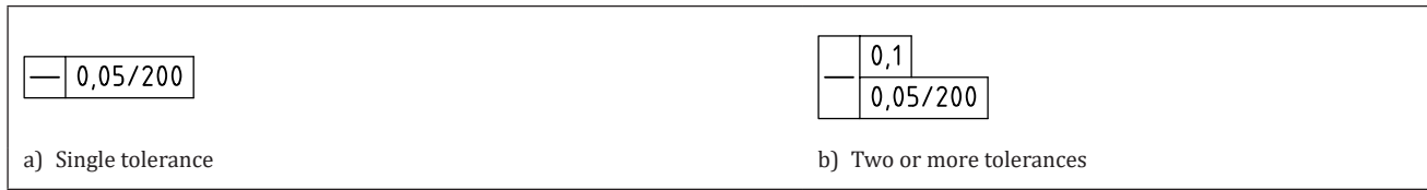
Figure 140 – Examples of tolerances of the same characteristic
