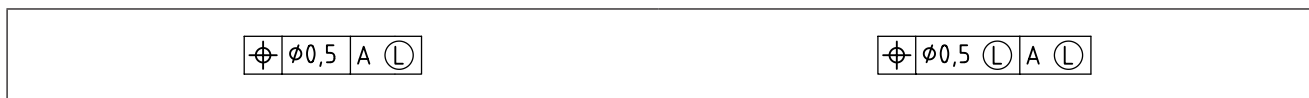
Figure 131 – Least material requirement applied to a datum reference in a tolerance indicator
