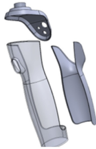
13 – SNAP HOOKS – HANDLE STEM COMPUND CURVE 3D SKETCH METHOD
