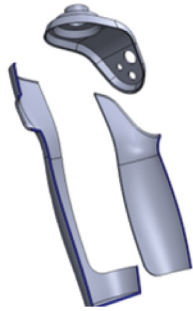
12 – WEBS + RIBS – HANDLE CAP CURVE DRIVEN PATTERN METHOD
